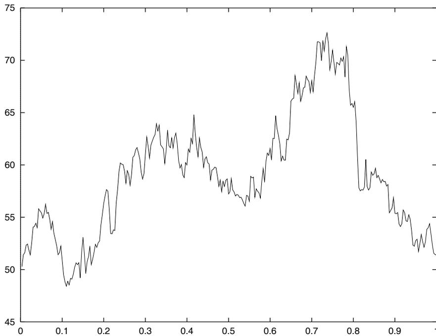
**Fig. 1.15.** Numerically approximated trajectory of Example 1.12 with  $a = 0.05X_t$ ,  $b = 0.3X_t$ ,  $\Delta t = 1/300$ ,  $X_0 = 50$
