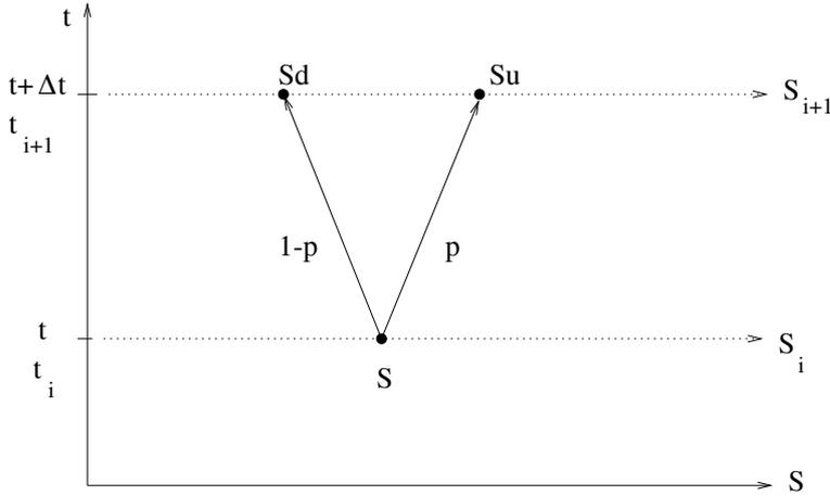
**Fig. 1.7.** The principle of the binomial method
