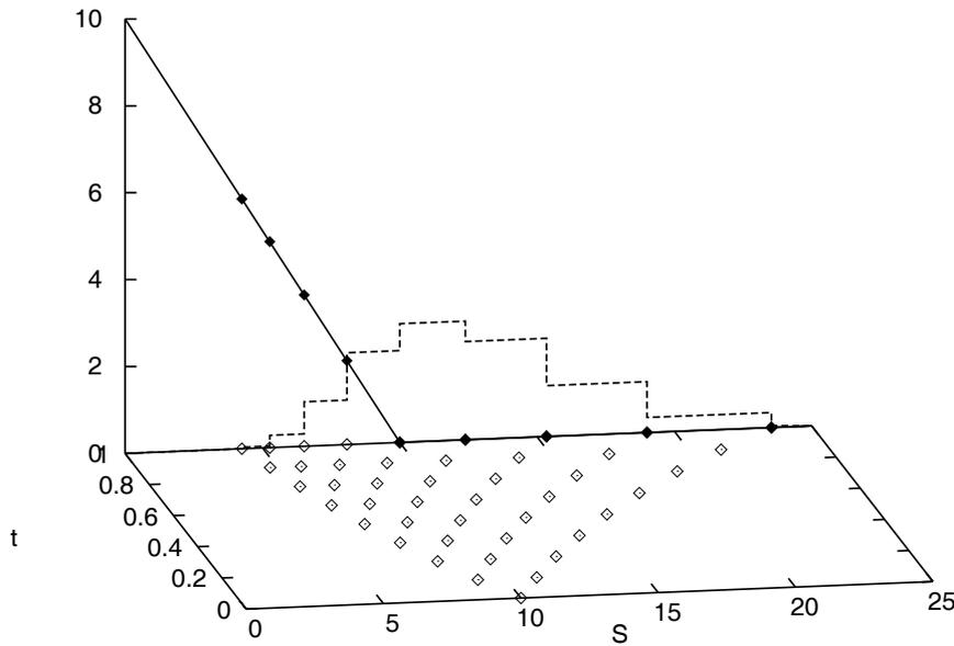
**Fig. 1.20.** Illustration of a binomial tree and payoff for Exercise 1.8, here for a put,  $(S, t)$  points for  $M = 8$ ,  $K = S_0 = 10$ . The binomial density is shown, scaled with factor 10.
