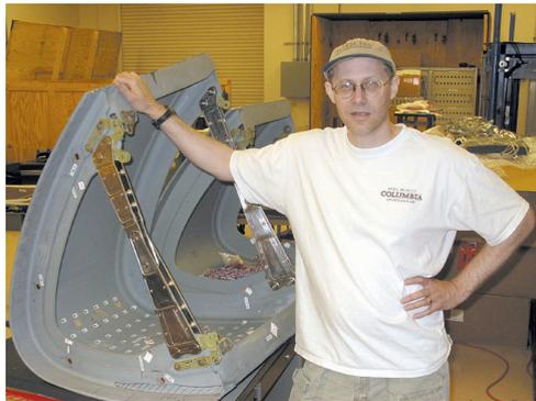
**Fig. 2.14** RCC Leading Edge with T-Seal.
