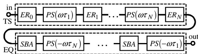
**Fig. 2.28** Transmission fiber span (TS) with elliptical retarders (ER) and DGD sections. Suitable equalizer (EQ) with Soleil-Babinet analogs (SBA; see text) and DGD sections, each of which may be accompanied by arbitrary differential phase shifts. © 1999 IEEE.
