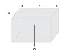
Counterclockwise torque > clockwise torque
