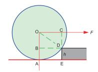
**1.42** Taking torque about D, the corner of the obstacle, (F)CD = (W)BD (Fig. 1.23)
